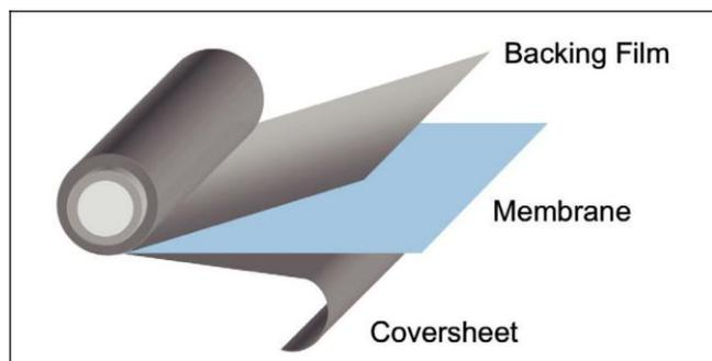
The 3.0-mil backing film facilitates transporting the membrane into automated fabrication processes, while the 0.92-mil coversheet protects the membrane from exposure to the environment during intermediate handling and processing. In addition, the coversheet (in combination with the backing film) eliminates rapid changes in the membrane's moisture content and stabilizes the dimensions of the membrane as it is removed from the roll.
